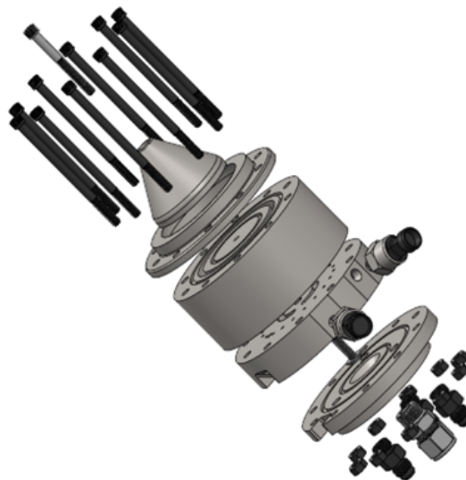
Figure 41: Exploded view showing modularity of the RDE combustor plate stack.
