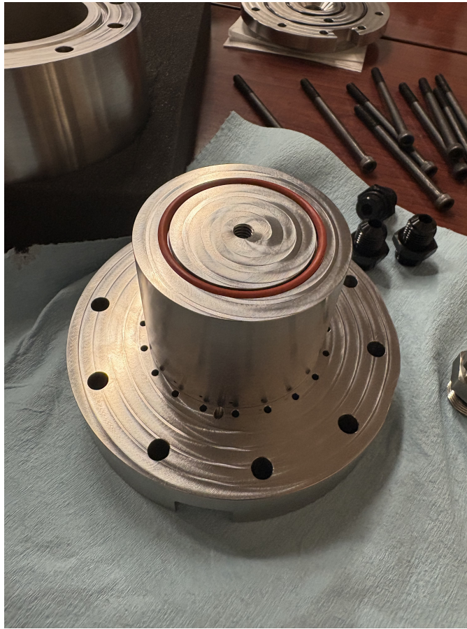
Figure 48: Old injector configuration with 20 jet-in-crossflow (JIC) pairs.
